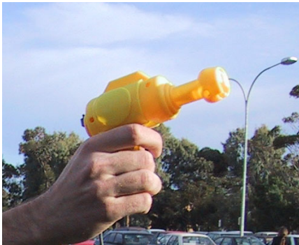
Figure 7 - USB mouse embedded into a children's bubble blowing toy, with switch and button attachments
