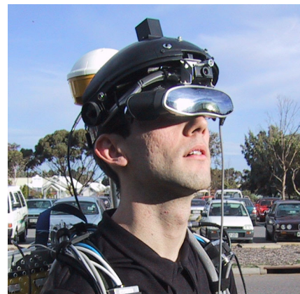
Figure 2 - User wearing a Sony Glasstron head mounted display, with attached video camera for AR overlay
