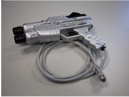
Figure 6 - Haptic feedback gun, embedded into futuristic looking children's laser gun toy (controller not shown)
