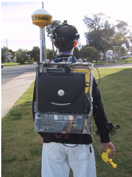
Figure 5 - Rear view of the Tinmith-Endeavour mobile backpack, with gun extension for ARQuake
