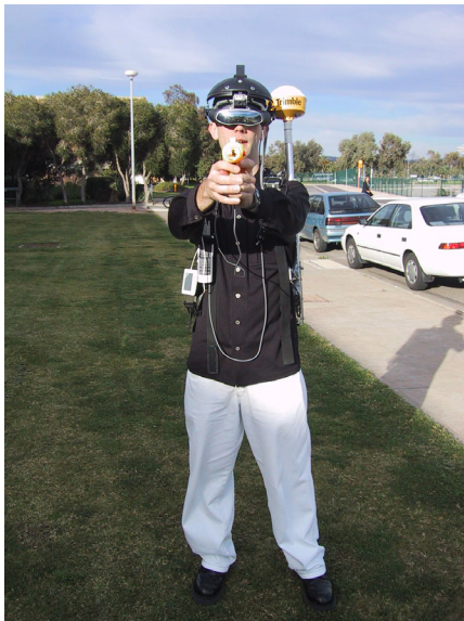
Figure 4 - Front view of the Tinmith-Endeavour mobile backpack, with gun extension for ARQuake
